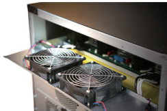
Redundant fan design enhances system reliability*
