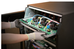
Swappable interior architecture for quick and easy maintenance*
